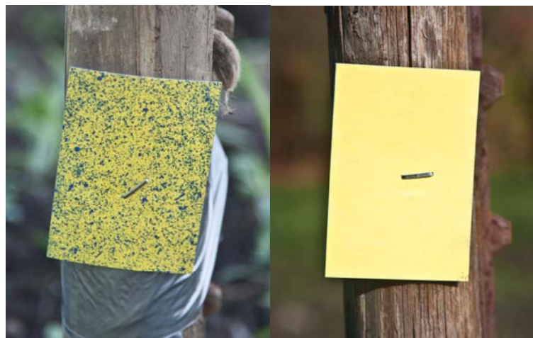
Figure 6. Water sensitive paper showing drift from the airblast sprayer (left photo) and the lack of any spray drift from the tunnel sprayer (right photo).
