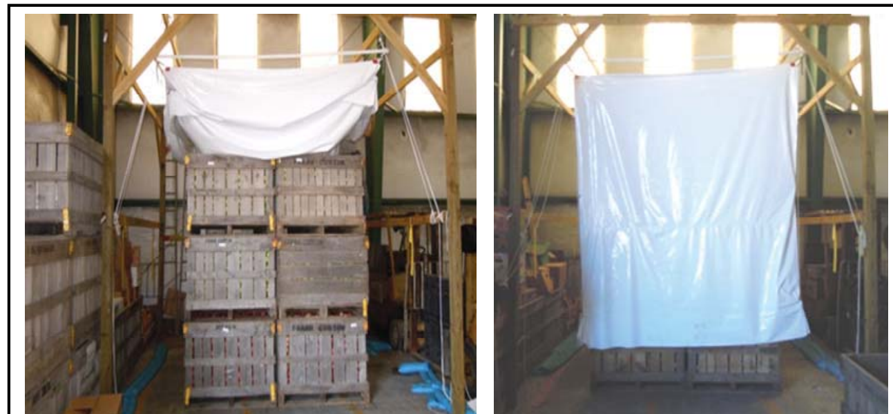
Figure 4. The Adjustable Apple Tent ( http://theblimpworks.com/ ) has a four bin footprint and can treat 4, 8, or 12 bins of fruit at a time. The tent is raised or lowered to minimize dead space and maintain the concentration of active ingredient at an effective level for the duration of the 24-hour treatment period. It is easily sealed around the base with a water bladder.
