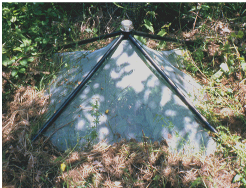
Pyramidal emergence trap used for the quantification of PC adult emergence after the application of either, the EPN Steinernema riobrave , or water (control). Trap dimensions: 1.1 x 1.1 yards at the base.
