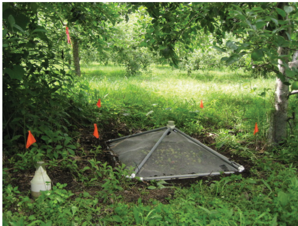
Figure 1. Depiction of the PVC enclosure (left) and pyramidal emergence cage (1 × 1 yards at the base) (center) used for the evaluation of entomopathogenic nematodes (EPNs) in the second study.
