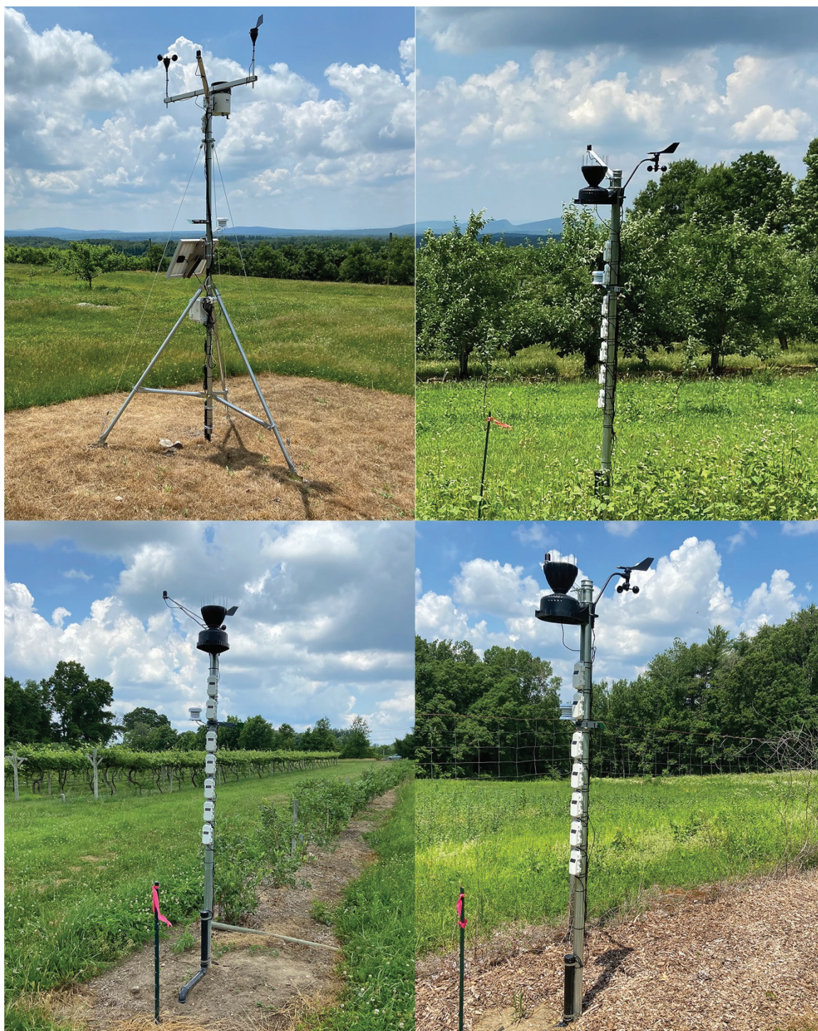
Figure 2. Four sites at the UMass Cold Spring Orchard showing the Onset RX3000 base station (North Hub, top left), and three different remote stations or “motes” (G, top right; Y, bottom left; X, bottom right).
