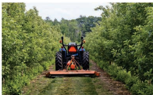
RAS-Rotary Mower. Ideal for mowing orchard rows.
