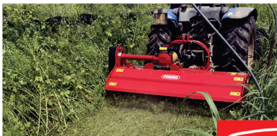
Shredder/Flail Mowers Ideal for chipping brush, managing field edges, handling cover crops
